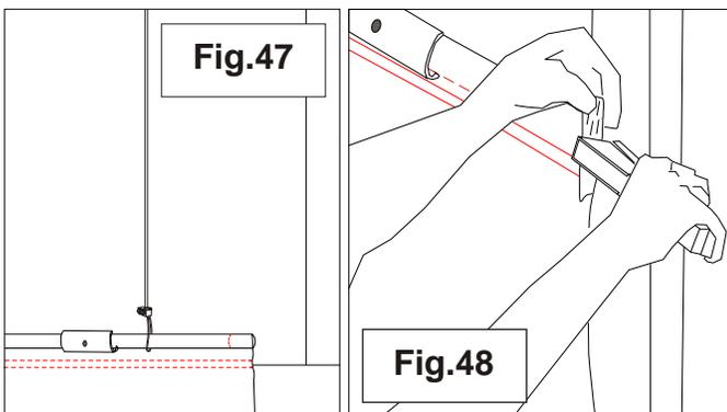
**48.** Fold over the material capping over the end of the rod. Staple closed as shown.
