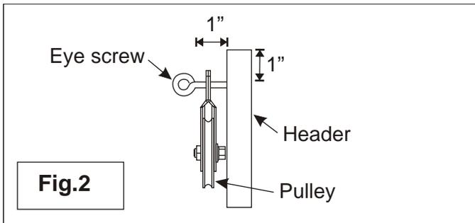
2. At these measurements screw in 2 1/2"x1/4" eye screws with a pulley hanging from the shaft. Screw it in until there is 1" of shaft remaining out from the face of the header (this allows the pulley to swing freely).
